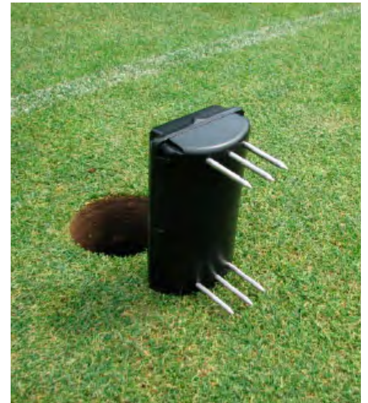
Figure 19. Moisture meters as part of an integrated irrigation management system (Courtesy of John J. Genovesi/Maidstone Club11).
